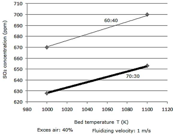
Figure 1. SO<sub>2</sub> emissions as functions of bed temperature at two particular air staging levels (the fluidizing velocity is fixed at 1 m/s, whereas the excess air is fixed at 40%)
