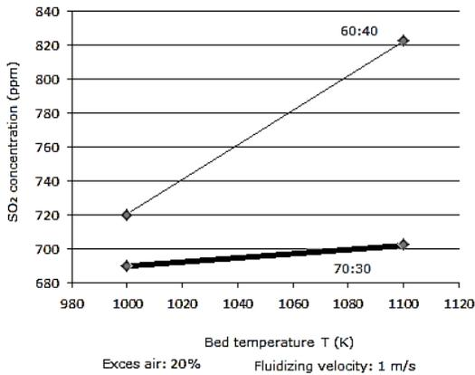
Figure 2. SO<sub>2</sub> emissions as functions of bed temperature at two particular air staging levels (the fluidizing velocity is fixed at 1 m/s, and the excess air is fixed at 20%).
