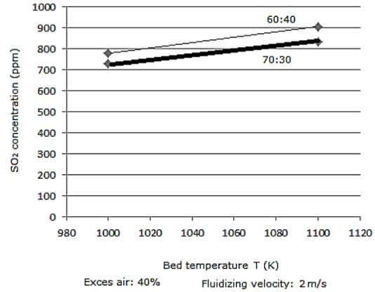
Figure 3. SO<sub>2</sub> emissions as functions of bed temperature at two particular air staging levels (the fluidizing velocity is fixed at 2 m/s, whereas the excess air is fixed at 40%)
