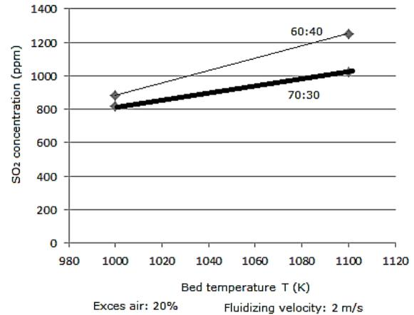
Figure 4. SO<sub>2</sub> emissions as functions of bed temperature at two particular air staging levels (the fluidizing velocity is fixed at 2 m/s, whereas the excess air is fixed at 20%)
