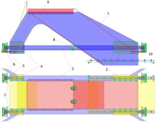
Figure 3. Chute for taking lignite samples
