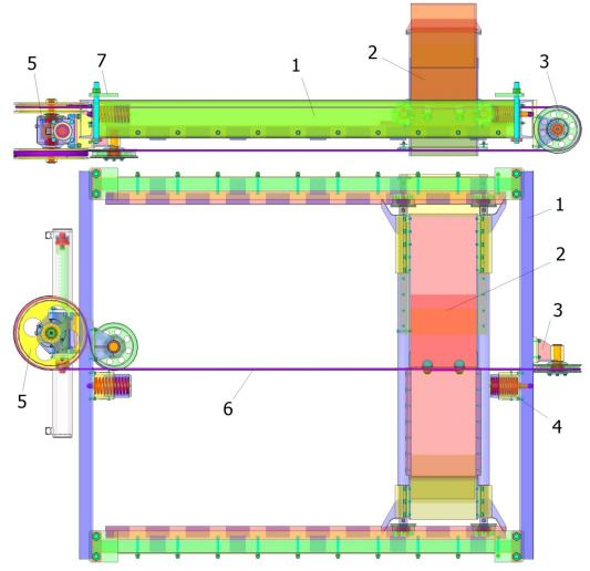
Figure 2. Device for taking the lignite sample from the discharge stream from the belt conveyor
