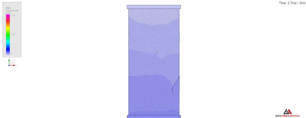
Fig.15 The moment of the appearance of the crack
