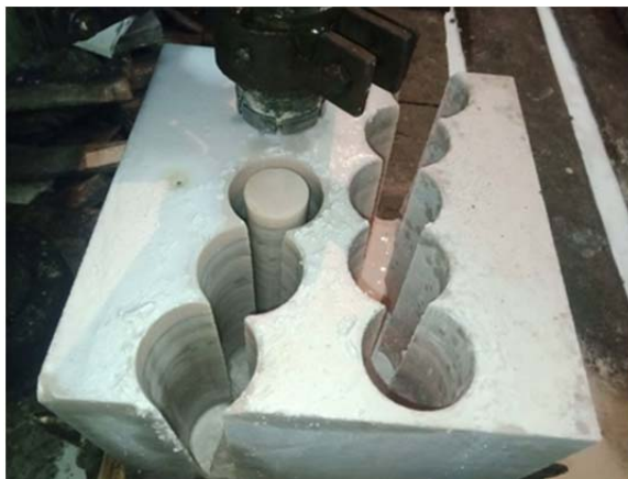
Fig.20 Obtaining the sample by coring – cracked specimen
