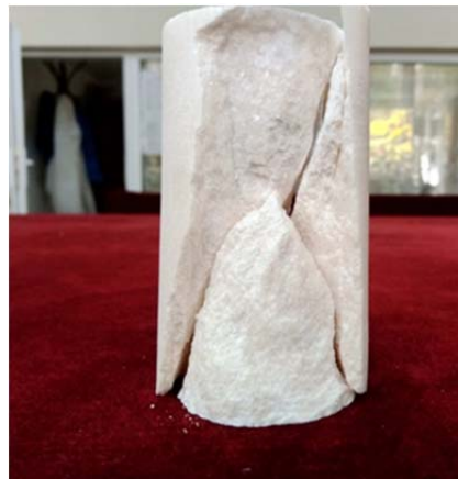
Fig.20 Obtaining the sample by coring – cracked specimen
