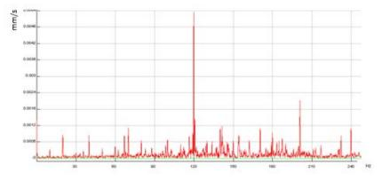
Fig. 7. Vibration FFT spectra on the fan of motor
