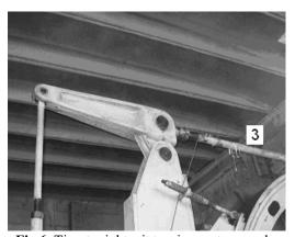
Fig.6. Tirant reight wit tension metres marks
