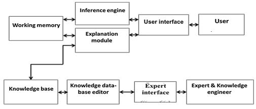
Fig. 3. Expert System components
