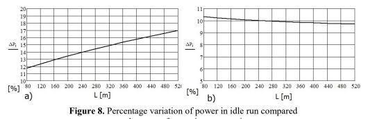
to the power for maximum capacity Figure 9 shows the variation of the acceleration when the belts starts, depending on the flow rate of the hauled coal and the belt length for the two cases, horizontal Figure 9.a and ascending at 12° in Fig. 9.b. The weight to be put to motion at idle run is 11,7 kN, and at maximum flow rate it reaches 334,1 kN for maximum belt
