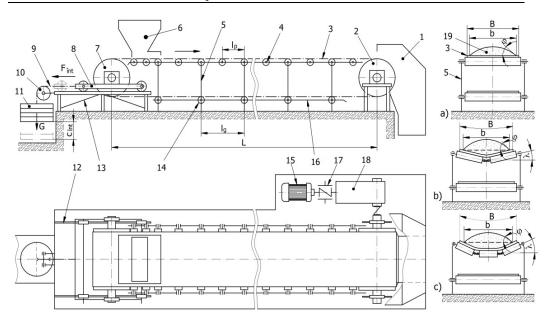
Figure 1. Construction diagram of a stationary roll belt conveyer
