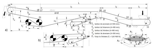
Figure 3. Diagram of the TMB conveyer with the inflection points along the route of the chain [driving drum, returning drum, stretching drum, dumping drum stretching force]
