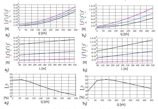
Figure 5. Variation of belt driving force function of the flow rate and length
