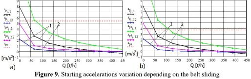
on the drum and on the coal sliding on the belt
