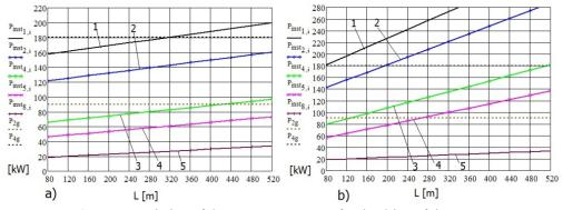
Figure 7. Variation of the necessary powers for the drive of the conveyer
