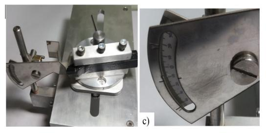
Figure 7. Measuring secondary angles of the lathe tool
