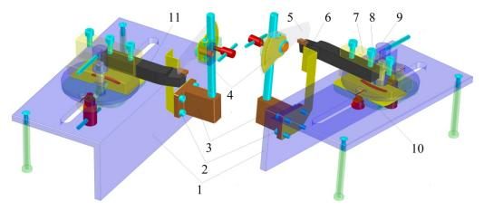
Figure 3. 3D model of the device for measuring lathe tool constructive angles
