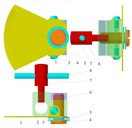
Figure 4. 3D model of the measuring unit
