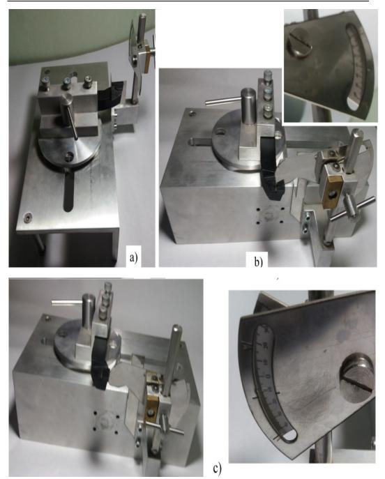
Figure 6. Measuring the main angles of the lathe tool
