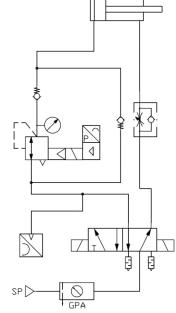
Fig.2 Pneumatic diagram for the velocity and force control of a single cylinder
