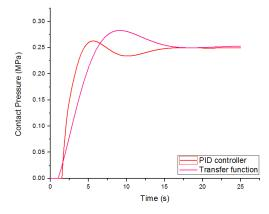
Fig.5 Step response of the system achieved by the open-loop transfer function and the PID controller
