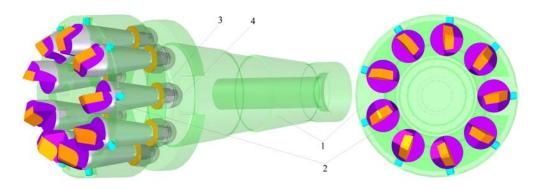
Fig. 4. 3D model of the Romascon milling head with the axes of the looks parallel to the body axis
