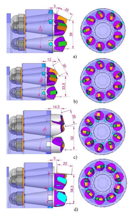
Fig. 5. Sharpening schemes for the Romascon milling heads with the axis of the tool parallel to the axis of the body of the milling head
