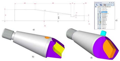
Fig. 3. 3D model of the tool reinforced with metal carbide plate and conical tail
