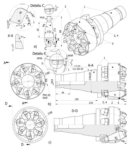
Fig. 1. The milling heads Romascon
