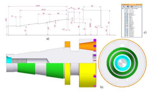
Fig. 2. 3D modeling of the body of the Romascon milling head with the axis if tools parallel to the axis of the body
