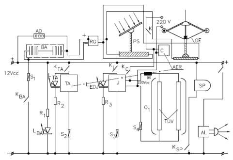
Fig. 5. Electrical scheme of the ozonozation device
