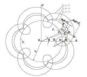
Fig. 1. Generation of the cycloid profile
