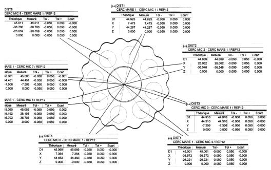
Fig. 4. The wheel holes centers circle's eccentricity.
