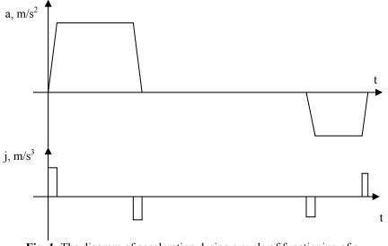
Fig. 1. The diagram of acceleration during a cycle of functioning of a mechanical system powered by an asynchronous machine
