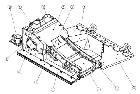
**Fig. 5.** Return station body of the TAGOR-260/750 type face conveyor: 1 – drive case; 2 – drive sprocket ensemble; 3 – left slider; 4 – right slider; 5 - lock; 6 –ejectors and ejector plate; 7 – superior lid; 8 – frontal lid; 9 - shield; 10 – anchorage beam; 11 – anchorage bottom; 12 - spur; 13 – secondary drive plate
