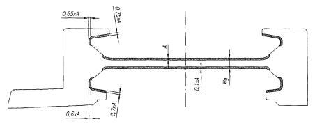
Fig. 9. Limits values of the slipping plate weare
