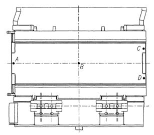
Fig. 8. Measurement points of the slipping plate thickness of Tagor conveyer
