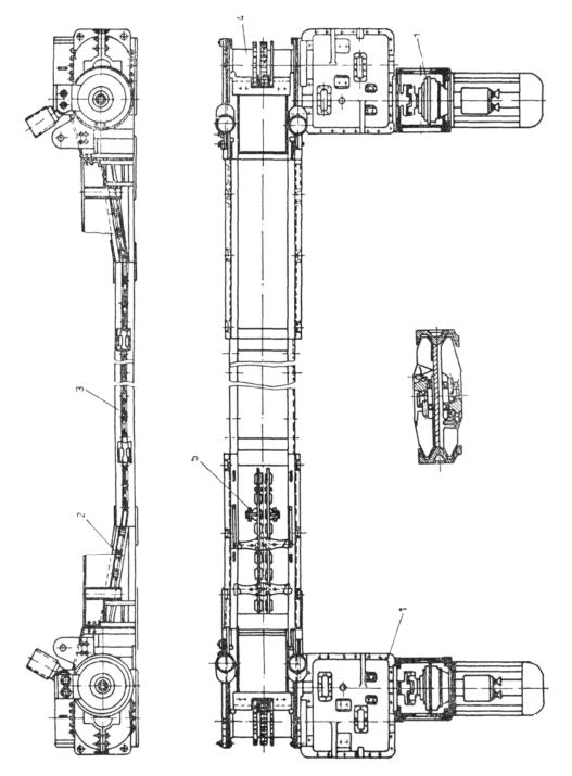
Fig. 1. TR-7A type push conveyor
