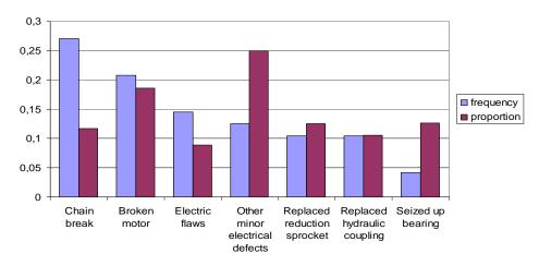
Fig. 7. Pareto diagram of TR-7A type conveyor failures
