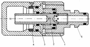
**Fig. 4.** Safety valve with nitrogen: 1- valve body; 2- piston; 3- valve sleeve; 4- sealing ring; 5- fixing cover
