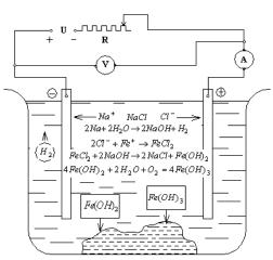
Fig.1. Processing diagram by electrochemical erosion.
