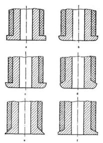
Fig. 3. Electrode-tools used to electrochemically deburr bore holes [12].
