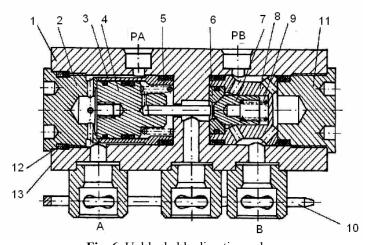
Fig. 6. Unblockable direction valve:
