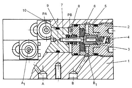
Fig. 7. Double deblockable valve of direction:
