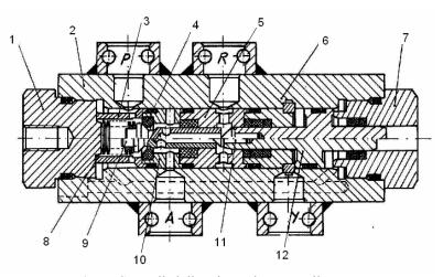
**Fig. 5.** Controlled direction valve normally open: 1- bored plug; 2- valve body; 3-spring guiding; 4- valve seat; 5-intermediary sleeve; 6- sleeve; 7- gland; 8- spring-disc; 9- control rod; 10- pass through sleeve; 11- sealing taper; 12- piston.
