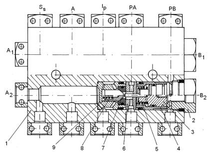
**Fig.8.** Double deblockable valve of direction: 1-valve body; 2 –piston cover, 3-piston with rod, 4-piston sleeve 5-come-back spring, 6-intermediary sleeve; 7-valve seat, 8-tapered valve; 9-pressure spring
