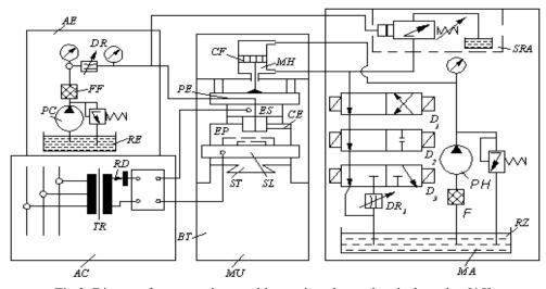
Fig.2. Diagram for processing machines using electrochemical erosion [15].
