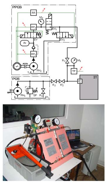
Fig. 2. Test stand for hydrostatic and cyclic pressure: hydraulic diagram and view
