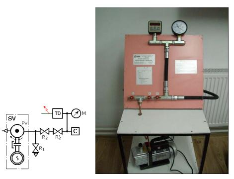
Fig. 3. Test stand for negative pressure: hydraulic diagram and view
