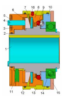
Fig. 10. 3D modelling of safety coupling with balls
