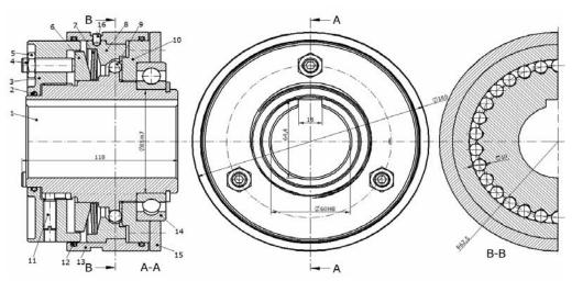
Fig. 11. Safety coupling with balls
