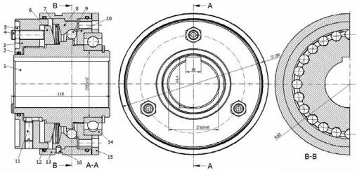
Fig. 4. Safety coupling with balls and trapezoidal canals
