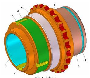
Fig. 5. Block a - wedge canal ( $18 \times 4,4$ ); b - bore hole Ø60 H7; c - thread M95 $\times 2$ ; d – slot for the head of the threaded pin; e - Ø100 e7 surface for the sliding of the pressure ring; f – slot for the ball  $\Phi 12$  with an 90° angle; g – canal for the elastic ring; h – mounting surface of the Ø85 m6 bearing.
