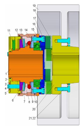
Fig. 3. General view of the assembly comprising the overload coupling with elastic coupler with brake washer
