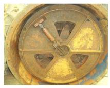
Fig. 2. General view of the friction safety coupling
