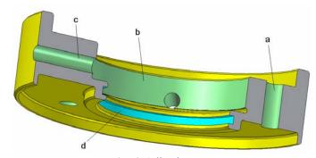
Fig. 6. Adjusting nut:
