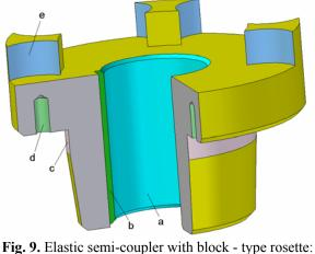
Fig. 9. Elastic semi-coupler with block - type rosette:
