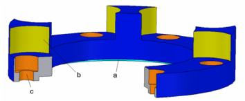
Fig. 8. Elastic semi-coupler with flange - type rosette: a – bore hole  $\Phi$ 130 H7 for centering on the bearing; b - contact surface with the elastic rosette; c - 8 holes  $\Phi 18/\Phi 11$ .
