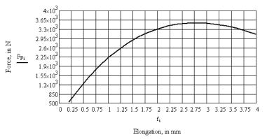
Fig. 14. Pre - tensioning feature of the disk springs on the coupling with balls and trapezoidal canals
