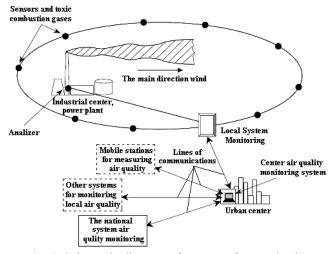
Fig. 4. Schematic diagram of a system for monitoring local air quality near a power plant.
